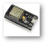
The ESP32s microcontroller is a series of low cost and lowpower system-on-chip microcontrollers with integrated Wi-Fi and dual-mode Bluetooth. The microcontroller is cheap with low-power consumption and a great number of pins. Evidently, with its varied features, IoT becomes easier when it comes to ESP-32. The continuously sensed data from the temperature sensor and heart beat sensors are transferred by the ESP 32 module to the web server.
