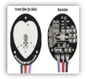
Heart beat sensor is designed to give a digital output of heat beat . When the heart beat detector is working, the beat LED flashes in unison with each heart beat. This pluse sensor is connected to the microcontroller directly to measure the Beats Per Minute (BPM) rate.Cattle have heart beat in the range of 48-84 beats per minute. If the heart beat is beyond this value it indicates stress or animal anxiety.
