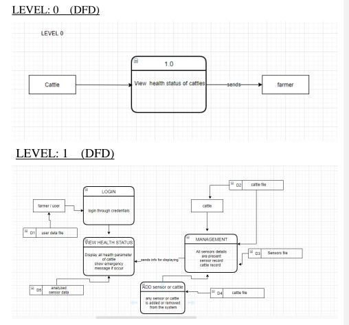
Here is our DFD of level 1. In this we have 4 data stores for storing user file, cattle file, sensor file, analyzed sensor file after analyzing. There are 4 processes as well for login, management of system, health status display and adding or removing sensor or cattle.
