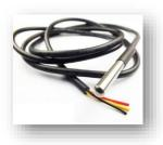
The DS18B20 is only one wire programmable Temperature sensor. It is used in hard environments. The constriction of the sensor is rugged and waterproof option making the mounting process easy. It can measure temperature from  $-55^{\circ}$ C to  $+125^{\circ}$ C. Each sensor has a unique address and requires only one pin of the MCU to transfer data so it a very good choice for measuring temperature at multiple points without compromising much of your digital pins on the microcontroller.
